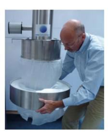
Figure 9-16: Cassette preloaded with liner
