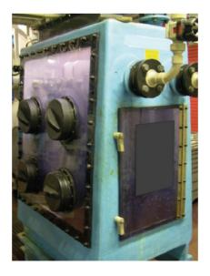
Figure 9-3: Glovebox with gloveport shields
