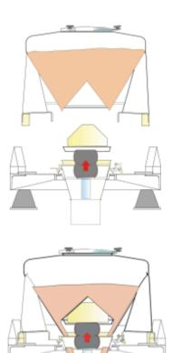
Figure 9-19: Matcon™ cone valve system
