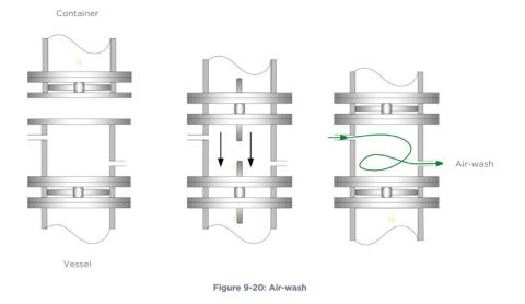
wash is introduced prior to the valves being uncoupled.
