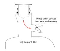
Figure 9-14: Contained connection of FIBC
