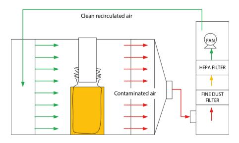
Figure 9-8: Horizontal laminar flow booth schematic (front view)
