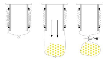
Figure 9-15: Continuous liner on spigot
