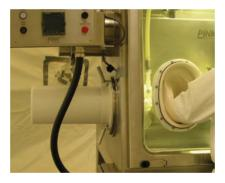
Figure 9-21(a): Beta canister docked to isolator
