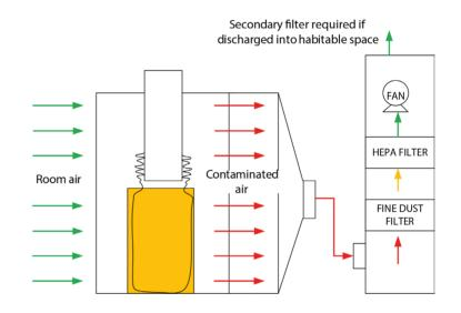
Figure 9-7: Horizontal laminar flow booth schematic (side view)
